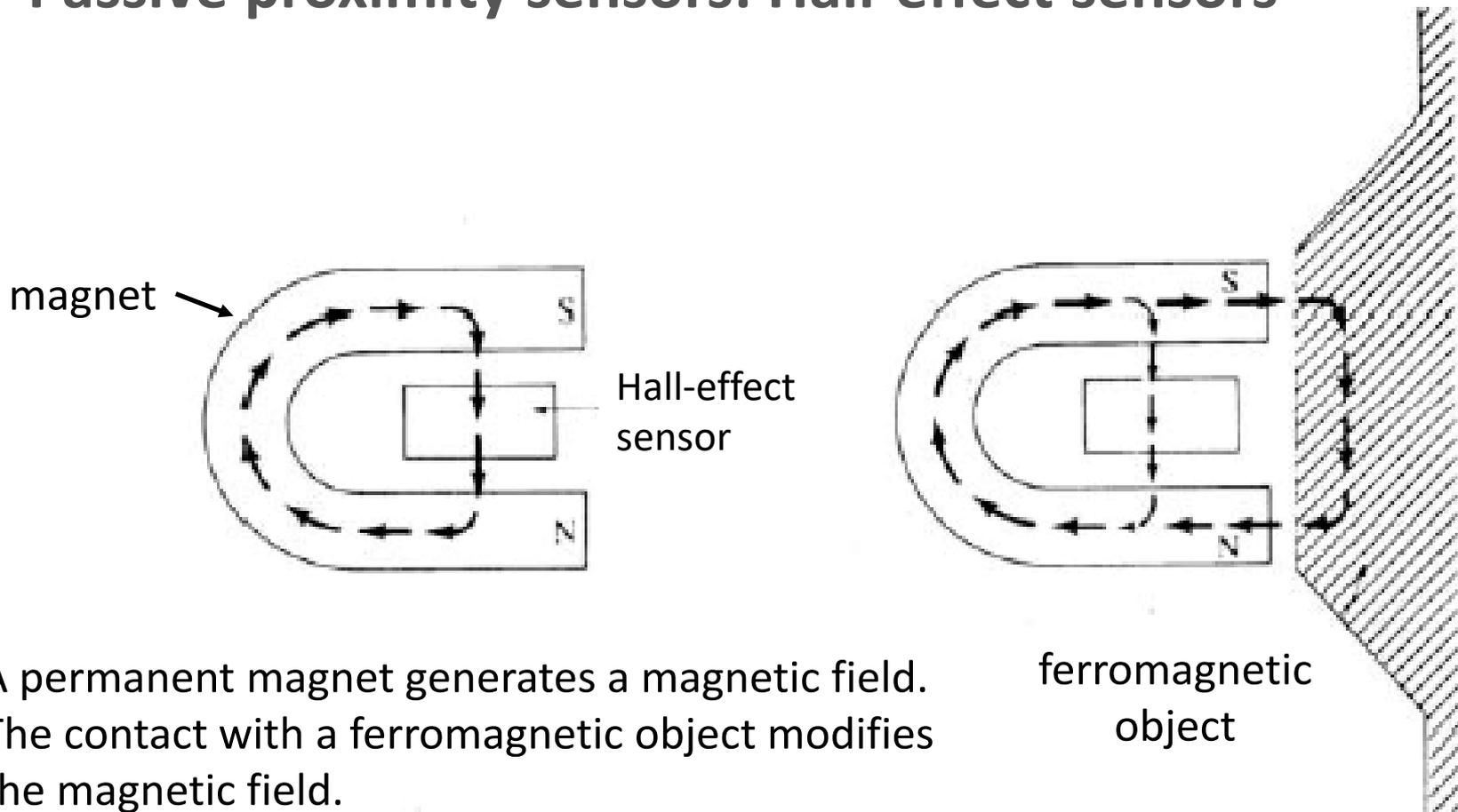
A permanent magnet generates a magnetic field. The contact with a ferromagnetic object modifies the magnetic field.
