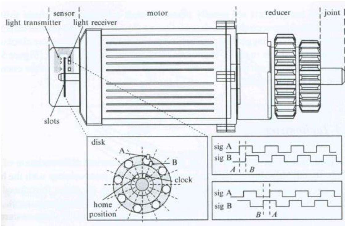
A and B are out of phase of  $\frac{1}{4}$  of cycle
