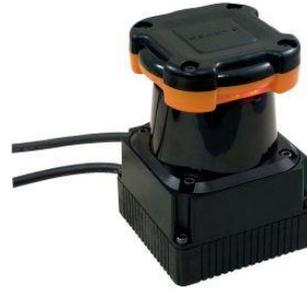
Measurement of range based on **time of flight**
