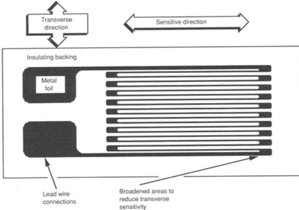
The sensor shape increases sensitivity in one direction
