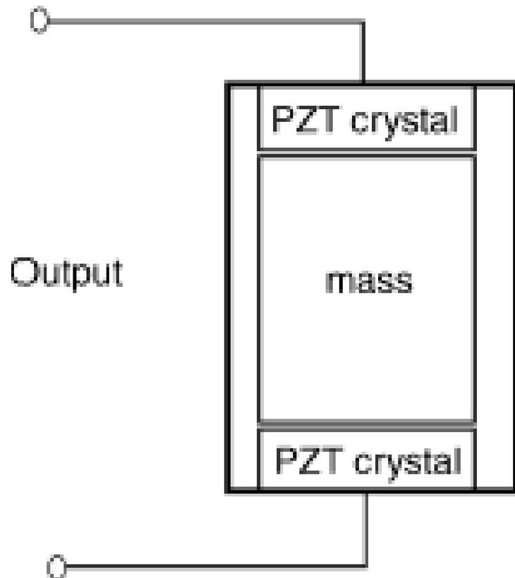
When a varying motion is applied to the accelerometer, the crystal experiences a varying force excitation ( $F = ma$ ), causing a proportional electric charge  $q$  to be developed across it.
