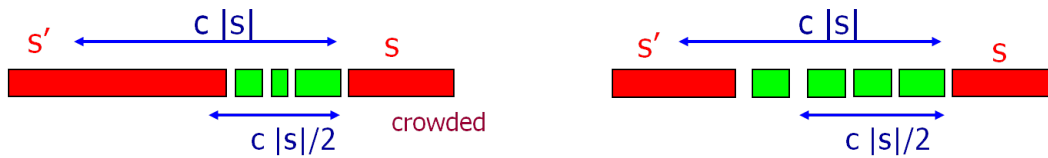
FIGURE 1.5: The two cases occurring in LPFC. The green rectangles denote the front-coded strings, and thus their FC-characters, the red rectangles denote the two consecutive copied strings.
