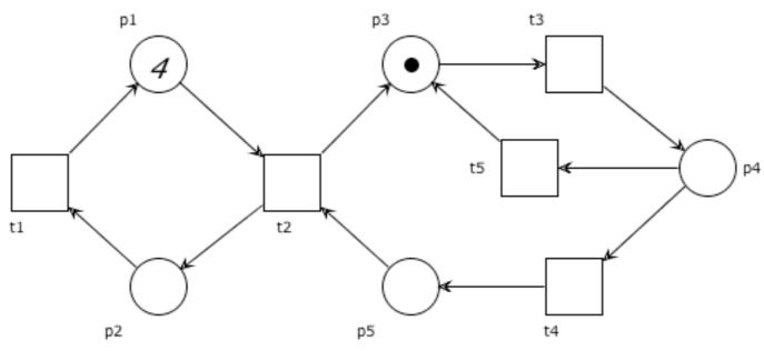
$$M_0 = [ 4 \quad 0 \quad 1 \quad 0 \quad 0 ] \qquad \sigma = t_3 t_5 t_3 t_4 t_2$$
