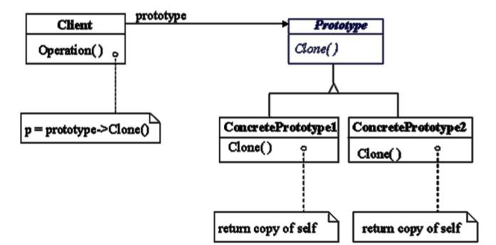
ol) - creates a new object by asking a prototype to clone itself.
