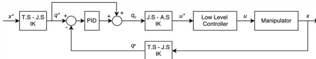
Closed-loop controller in joint space
