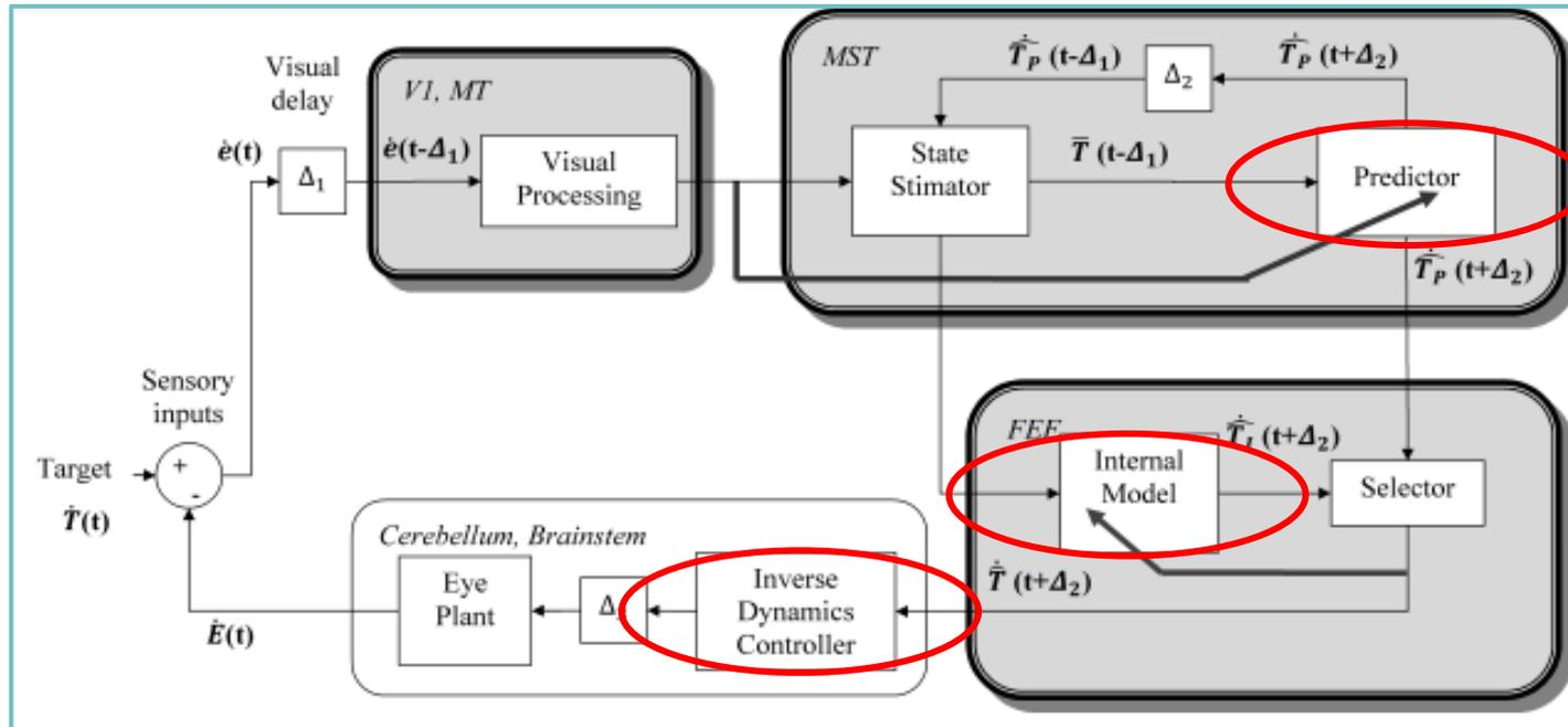
This circuit is based on Shibata and Schaal's model (Shibata 2005) of smooth pursuit and consists of **three subsystems**:
