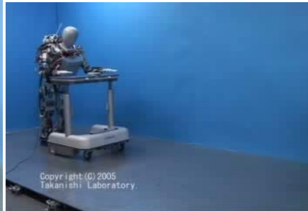
WABIAN testing the Walking Aid Robot for Elderly developed by HITACHI (WABOT-HOUSE Project, Gifu Prefecture)
