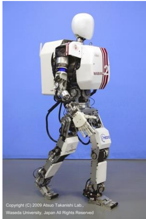
2-DOF model for the waist mechanism allowing knee stretch walking
