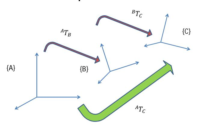
$$^{A}T_{C} = ^{A}T_{B}^{B}T_{C}$$
