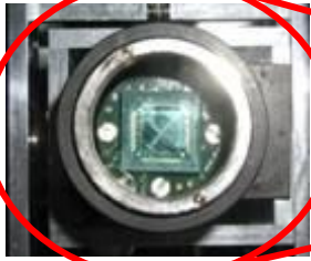
Retina-like Giotto cameras by the University of Genova, Italy
