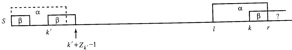
Figure 1.5: Case 2b. The longest string starting at k' that matches a prefix of S is at least |\beta| .
