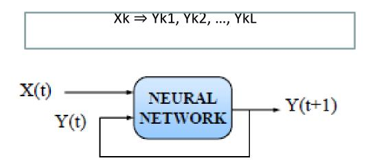
A recurrent neural network (RNN) is a class of neural networks where connections between units form a directed cycle. This creates an internal state of the network which allows it to exhibit dynamic temporal behavior.
