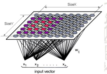
The SOM defines a **mapping** from the input data space spanned by  $x_1..x_n$  onto a one- or two-dimensional array of nodes. The mapping is performed in a way that the topological relationships in the n-dimensional input space are maintained when mapped to the SOM. In addition, the local density of data is also reflected by the map: areas of the input data space which are represented by more data are mapped to a larger area of the SOM.
