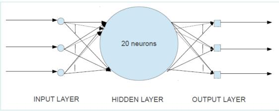
The network has one hidden layer of 20 units. It takes as input the head orientation (ν,φ,ψ) and as output the neck joints angles (θ1, θ2, θ3).
