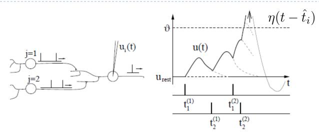
When the membrane potential exceeds a threshold the dynamics changes:
