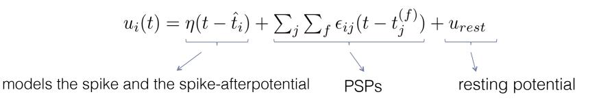
If the membrane potential reaches the threshold from below then fire!
